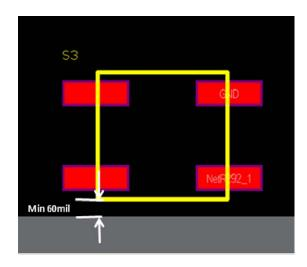
10. Components placed on the solder side (bottom side) should keep at lease 5mm (200mil) away from the leads of PTH components.
