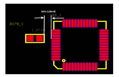
7. For SMT connectors, keep the height of the connector as the minimum clearance to the other components. For example, if the connector is 3.5mm high, then please keep at lease 3.5mm between this connector to adjacent components.
