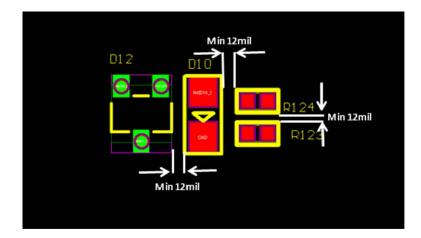
4. For these wave solder PCB design, keep at least 1.2mm (47 mil)(PCB moving axis) and 0.8mm (32 mil)( vertical axis) between chip ,DIP or SOT parts. For high profile chip components (like tantalum capacitor), increase the distance to 2.5mm (100 mil).
