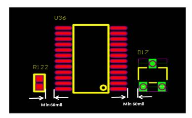
3. For these re-flow solder PCB design, please keep at lease 0.3mm (12mil) between chip, DIP or SOT components.
