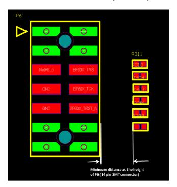
8. Leave at lease 2mm (80 mil) from component to the shield soldering pad (metal shield is quite normal used in wireless product designs).
