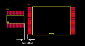
2. Keep at least 1.5mm (60mil) between QFP or SOP components to chip, DIP or SOT components.
