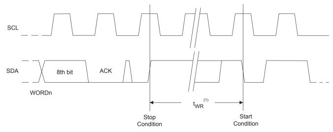
Notes: 1. The write cycle time t<sub>WR</sub> is the time from a valid Stop condition of a write sequence to the end of the internal clear/write cycle.
