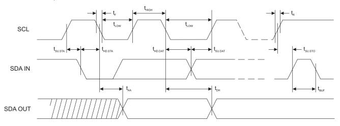
Figure 5-3. Write Cycle Timing
