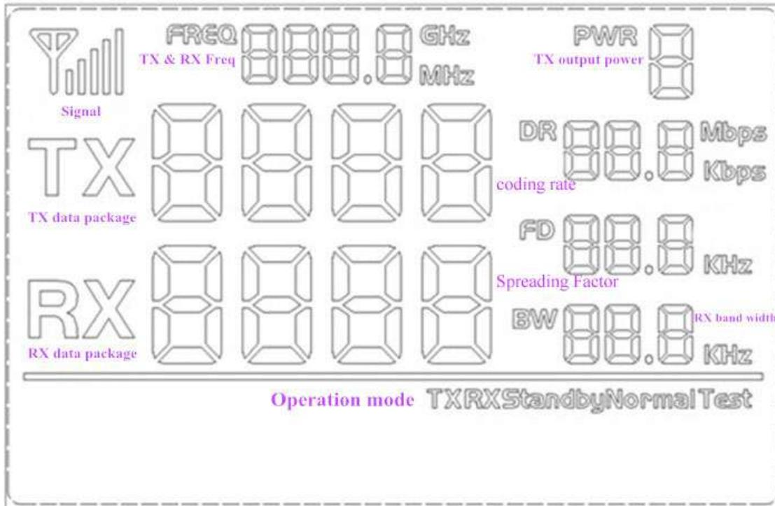
Users can set the parameters of the RF module such as working mode /frequency / transmitter power / transmission data rate through the buttons, and measure the wireless communication distance.
