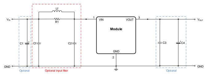
The 17950x36 partially integrates both the input and output capacitors. It is also recommended to use a  $10\mu\text{F}$  input capacitor C2 for high impedance input wires or traces and  $22\mu\text{F}$  output capacitor C3 for applications where a low output voltage ripple is required.
