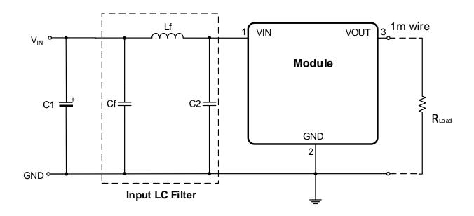
Bill of Material of the Input LC Filter (VIN = 24V, VOUT = 3.3V & 5V, IOUT = 500mA)
